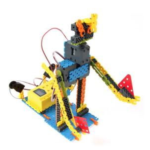
Input: Touch sensor Output: DC motor, Servo motor Work: Hanging up right/left hands, Head spining
