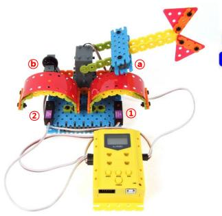
This Twinkle Robot model is for studing the Servo motor programming.
